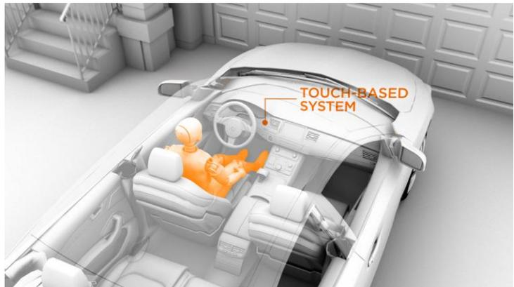
signal when the driver is seated. When the driver presses the stop/start button or wherever the sensor is located, the driver completes the loop and confirms that he or she is the person touching the button. If anyone not in the driver seat presses the button, the circuit will not be closed and the alcohol measurement will not be considered valid.
